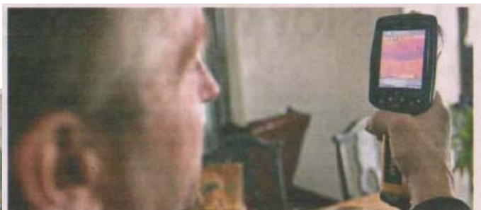
Dave Bunn from Green Build Technology uses an infrared camera to check the thermal integrity of a home during a home energy audit. Ben Woloszyn/Boomerang photographer
