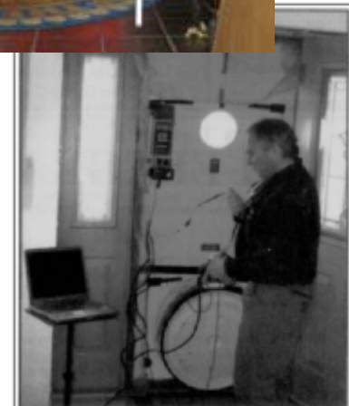
Dave Bunn, owner of Green Build Technology from Laramie, performs a blower door test on the second house built by students in the EWC Construction Technology program. The program uses environmentally-friendly building practices such as Energy Star and LEED. Photo: Jerry Abbott
